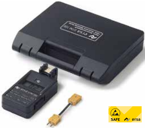
The DTM 100 is equipped with a patented sensor unit (K-type) with sensor wires made of chromel and alumel. It provides exact temperatures of even finest soldering tips.
