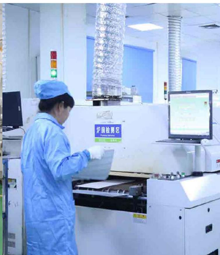
*Inspection on reflow oven first batch*
