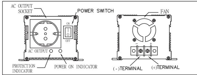
WHEN CONNECTED TO ANY APPLIANCE, BE SURE TO TURN ON INVERTER FIRST AND THEN, TURN ON THE POWER SWITCH OF THE APPLIANCE
