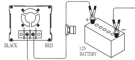
DURING OPERATION, WHEN THE POWER SWITCH IS ON, IF POWER ON INDICATOR IS NO LIGHTED, PLEASE CHECK THE FUSE IN THE BATTERY CORD. IF THE FUSE IS SPOILT, FOR REPLACEMENT, USE THE SAME CURRENT FUSE.
