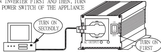
CAUTION: DO NOT REVERSE INPUT. USE RED BATTERY CORD TO CONNECT (+) OF A 12V DC BATTERY TO (+) TERMINAL AND THEN, USE BLACK BATTERY CORD TO CONNECT (-) BATTERY TO (-) TERMINAL.
